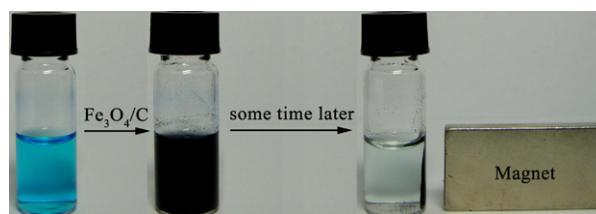
Fig. 8. Photographs of \text{Fe}_3\text{O}_4/\text{C} composites adsorption behavior and magnetic separation phenomenon. Blue solution is MB solution, after mix with \text{Fe}_3\text{O}_4/\text{C} composite a few hours later, magnetic separation by an external magnet can obtain a clear solution.
